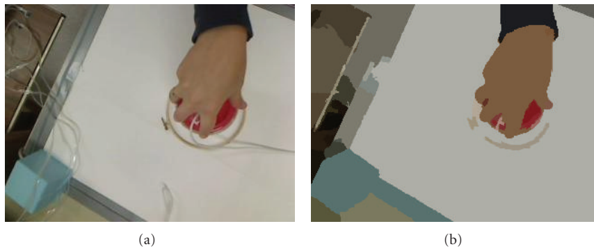
FIGURE 4: Example of the mean shift segmentation algorithm [31]. (a) Sample image from database used in this article. (b) Segmentation of (a) using the EDISON system [32].
